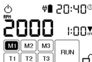
Touch the M1 key on the display. Use this button to set application time No.1. Then press the button showing the application time (on the right in the middle of the display time arrow OFF) and then the display with numerical options will appear:
