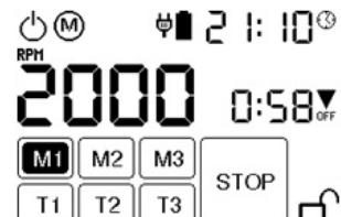
If the user wants to stop the program before the remaining application time has elapsed, press the STOP button on the display.
