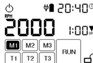
The RPM and application time below are set in the factory settings of the device memory:
