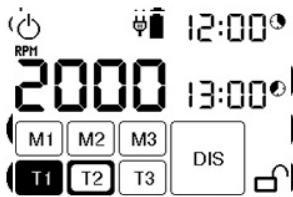
After the time interval of 5 minutes elapses, during which the PrimerCube has not been active, the device switches to the STANDBY mode, i.e. the sleep mode. In this off mode, the internal battery can be maintained fully charged for about 1 month. Preset programs are saved in the device's memory because the EEPROM memory does not depend on the battery charging activity.
