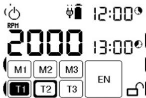
The deactivation of this function – timer – can be set by pressing the DIS button. After deactivation, the T1 value is displayed without a border in a smaller black cube.
